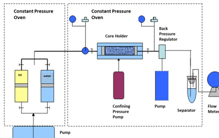
Figure3. Schematic of the apparatus
