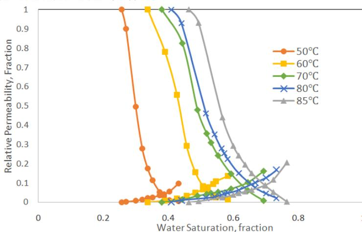
Figure 4. Water-oil relative permeability curve under different temperature (1000 mD group)
