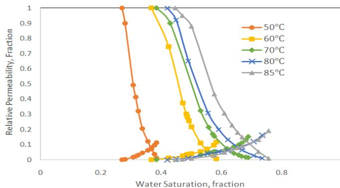
Figure 5. Water-oil relative permeability curve under different temperature (300 mD group)
