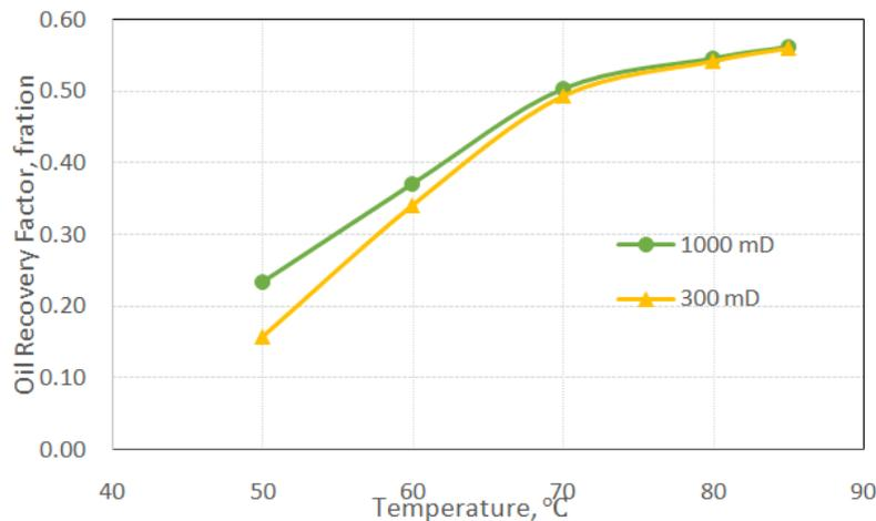
Figure 6. Oil recovery factors of 2 groups of displacement experiments
